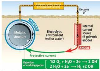
*Figure 2. Principe of cathodic protection.*
