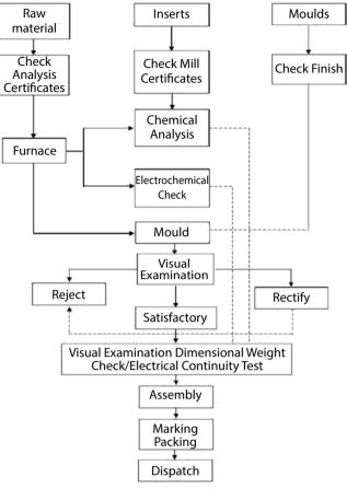
Figure 3. Procedure of sacrificial anode production.
