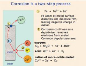
Figure 1. Electrochemical corrosion of iron.
